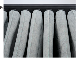
Tapered pocket design eliminates pocket-to-pocket contact ensuring full use of media area and reduced resistance to airflow for energy saving performance.
