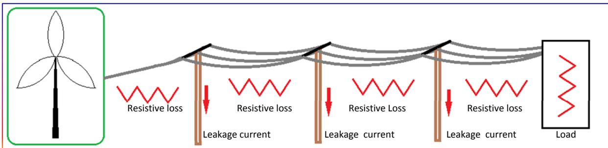
Since the relationship between Voltage and Resistance is exponential a 10% drop in voltage results a 19% loss in available energy; if during an extreme peak-demand we lose half of the voltage due to line-losses, the power that is available at the end of the line would only be 25%, and if this voltage dropped by 68% only 10% of the original energy would still be available.
